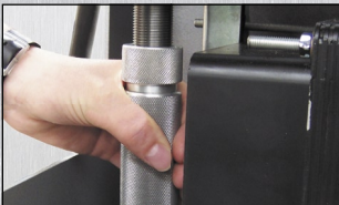
Easily adjustable gap limitation of the upper arm.
